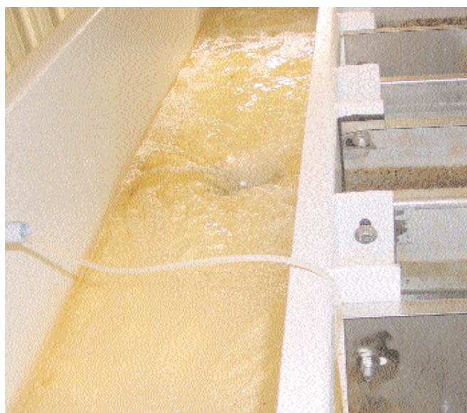
In a dissolved air flotation machine, particles in the waste water process coagulate and expand. Sludge forms and moves to rendering, and pipes transport the water to the lagoon.
